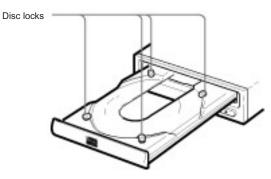
**4** Gently push the tray or press the eject button to close the tray. The drive will begin reading the Table of Contents (TOC) data when it accepts the disc. The busy indicator lights up in amber while the drive is reading the TOC.
